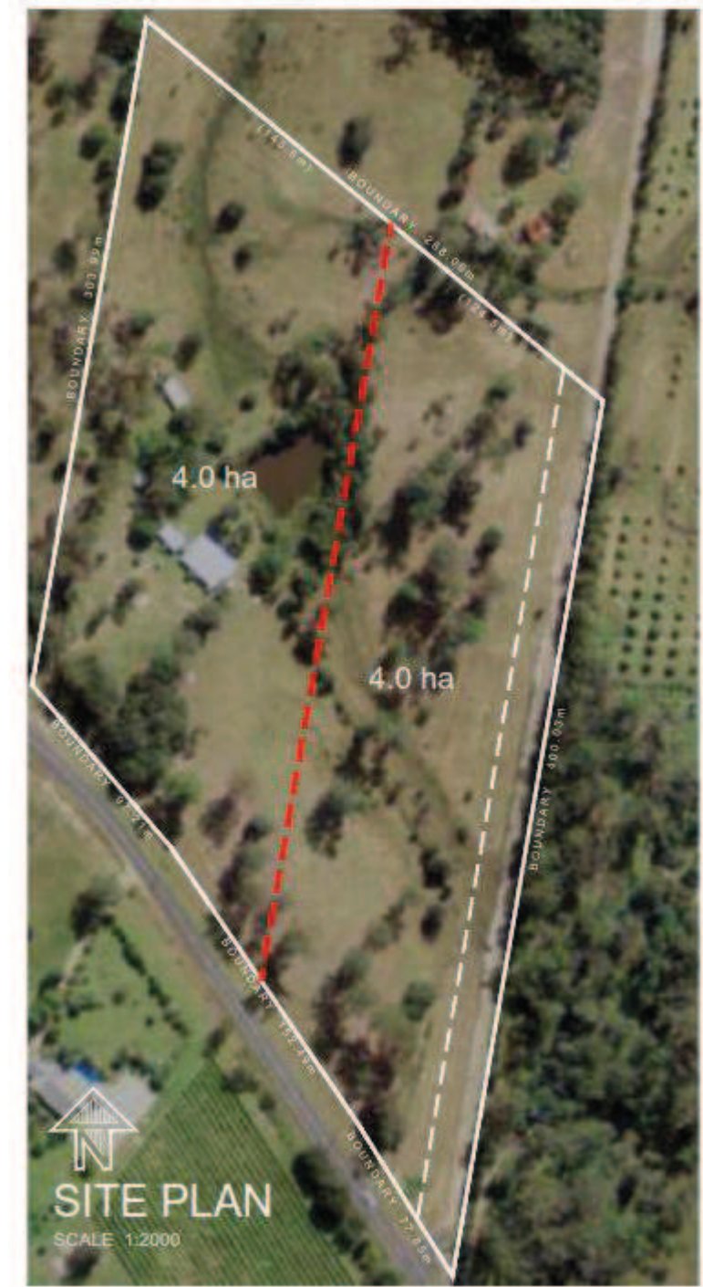
Option A – North South subdivision boundary for 2 x 4ha lots (subject to survey)
